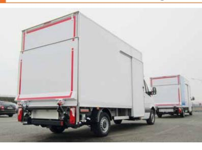
The DH-LSP4 is equipped with a compact lift frame and **very short lift arms**.
