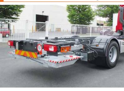
The DH-SM.15 is the **lightest of the conventional slider lifts** with single fold platforms. It is equipped with a compact lift frame and short lift arms, in order to **minimize the required overhang**. As a consequence, it forms a modern and lighter weight alternative to the short overhang lift DH-SMP.20 in 1500 kg execution.
