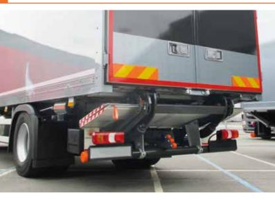
The DH-RM.20 is equipped with a robust lift frame, a wide arm center and 2 lift cylinders. Hence it serves the **heavy-duty end of the fold-away lift market**. It is equipped with a wedged platform, offering a level ride from the vehicle floor to the ground (and vice versa), including **automatic tilt at ground level**.
